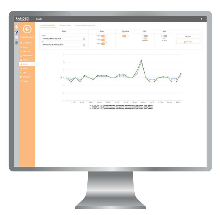
Levey-Jennings charts are easily generated, providing an instant, visual indication of test system performance over time. The ability to conveniently combine multiple instruments, analytes, QC lots and labs on a single chart allows for comparative performance assessment and immediate visualisation of any ongoing or emerging trends. Customisation in this way will improve troubleshooting capabilities, enabling you to quickly identify whether an issue is unique to a particular test or
