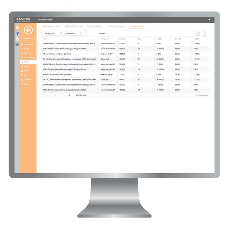
Designed to quickly and easily identify assays with a high percentage of errors, the new exception report provides an on screen summary of the number of QC results for each individual assay and control lot that fall within the following categories: <2SD, 2-3SD and >3SD.
