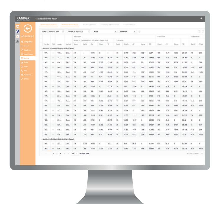
Displays statistical metrics including Bias%, Sigma and Total Error (TE) for each test alongside those for your chosen peer group. The Bias% provides an indication of your laboratory's performance compared to the Peer Group Mean, while TE gives an indication of the overall error within a test system, taking into account both imprecision and inaccuracy.
