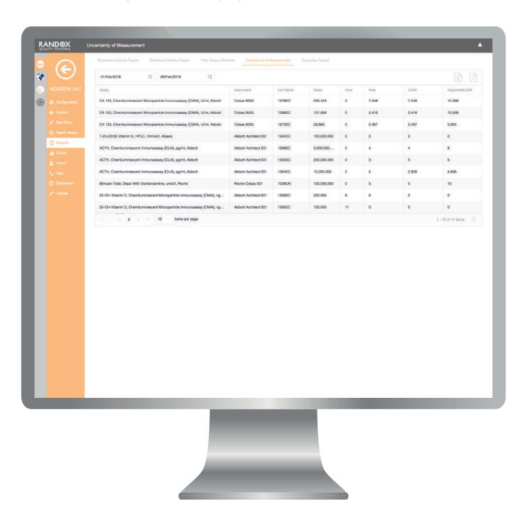
The unique Uncertainty of Measurement report displays the UM of all QC tests currently in use, helping you to meet ISO 15189:2012 requirements. To calculate UM, simply enter the SD or Standard Error of the Mean (SEM) of the intra assay precision for each test and level of control. Based on performance history,
